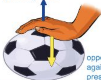
air in a ball opposes a pressure.
