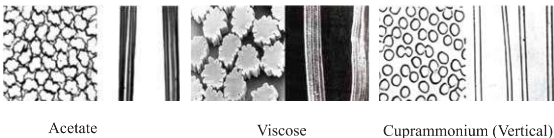
Fig. 6.02 : Shapes of rayon fibers under microscope
