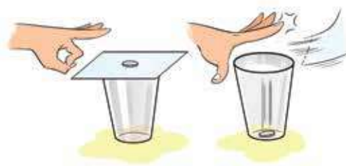
Fig.10.01: Experiment of inertia
