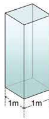
Figure 5.06: The pressure of air comes from the weight of the air column.
