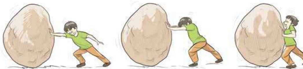
Figure 5.01: Pressure depends on the area through which force is applied
